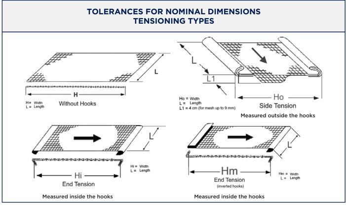
For **SIDE TENSION**, the tolerances described below are based on the expectation of a 40 mm clearance in relation to the screenwalls
